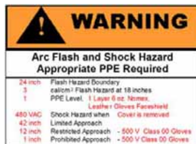
Figure 4.5 Arc flash and shock hazard warning sign at a workplace
