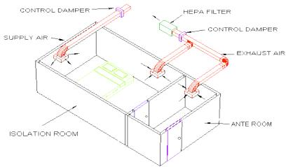
Figure 4: Negative-pressure isolation room
