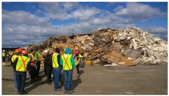
Construction and demolition waste after a rough sort, before milling and screening October 2014 (Photo by W. Mabee)
